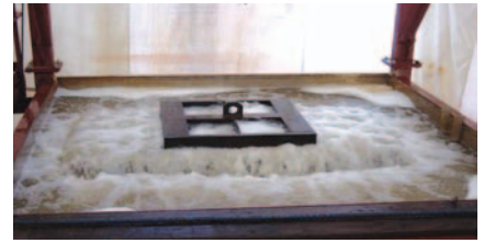
d. Bubbling and aeration under pressure
