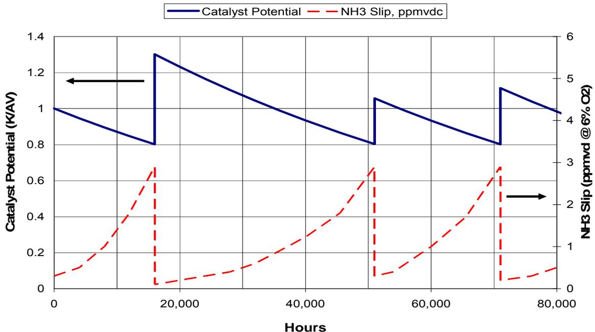
Figure 3 Catalyst Management Plan 16,000 Hour Design Life (2 + 1 Layer)
