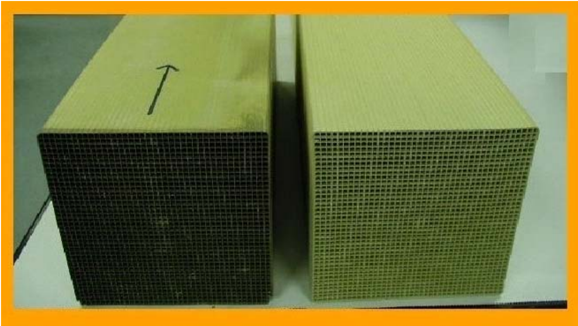
Figure 6: Photograph of SCR Catalyst Samples Left: Exposed Sample from SMR Service Right: Fresh Sample
